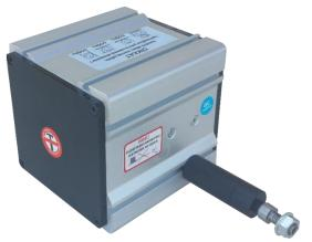
The AWP series are wire potentiometric position transducers that turn a linear motion into a resistance variation. They are made of a precision rotating potentiometer operated by a, winding or unwinding, stainless steel wire. Optionally other stroke lengths, cable length and socket connector can be requested.
